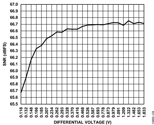
Figure 35. SNR vs. Clock Amplitude (Differential Voltage), f_{IN} = 155.3 MHz
