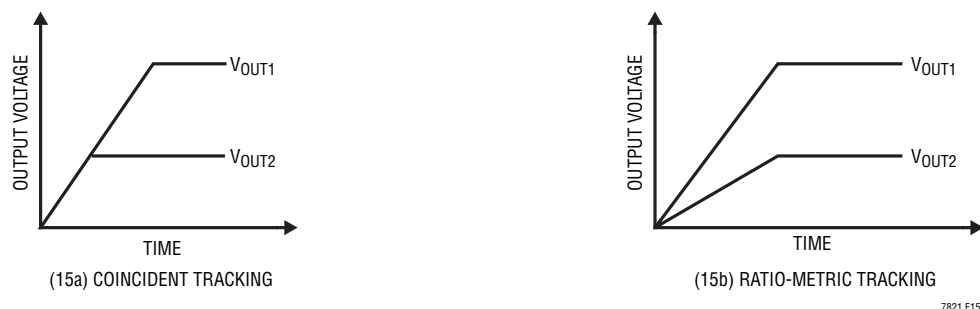
Figure 15. Two Different Methods of Output Voltage Tracking
