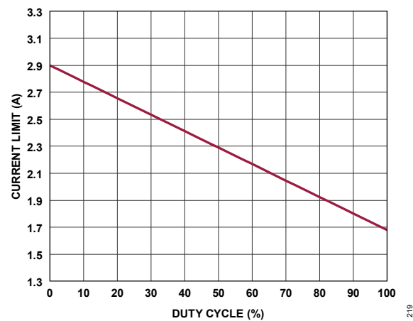
Figure 24. Top MOSFET Current Limit vs. Duty Cycle
