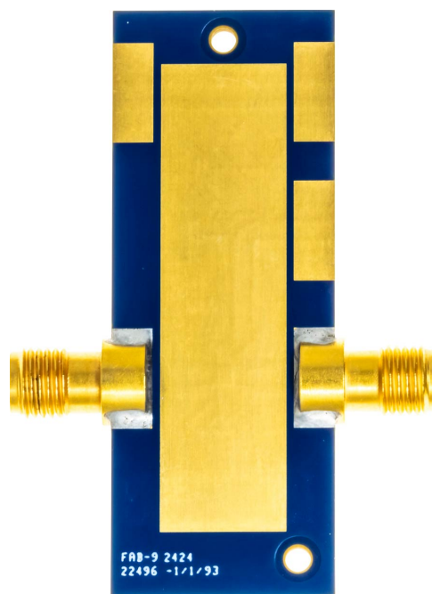
Figure 2. ADL8108-EVALZ Secondary Side
