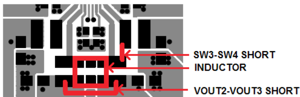
Figure 6. Combined 3A Regulator Inductor Placement and Connections
