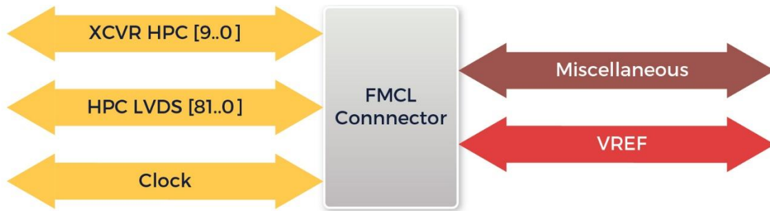
Figure 2-15 Interfaces connected through the FMCL connector
