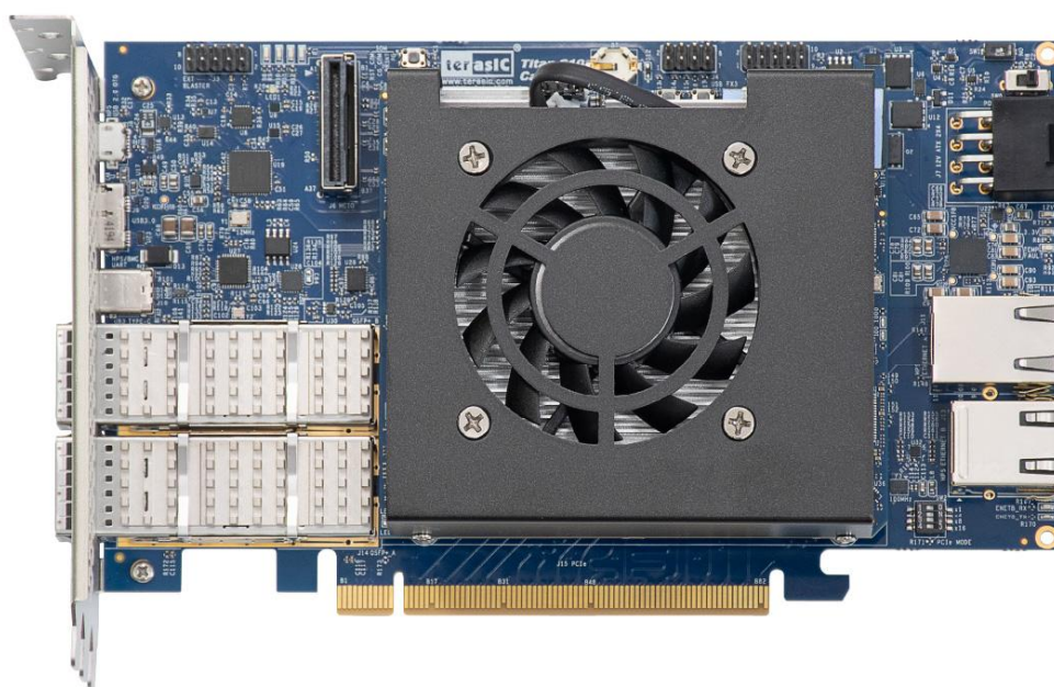
Figure 1-8 Titan S10 SOM connects to the carrier board
