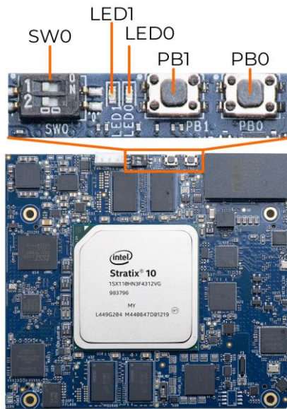
Figure 2-6 Position of all the user LEDs/Switches/Buttons
