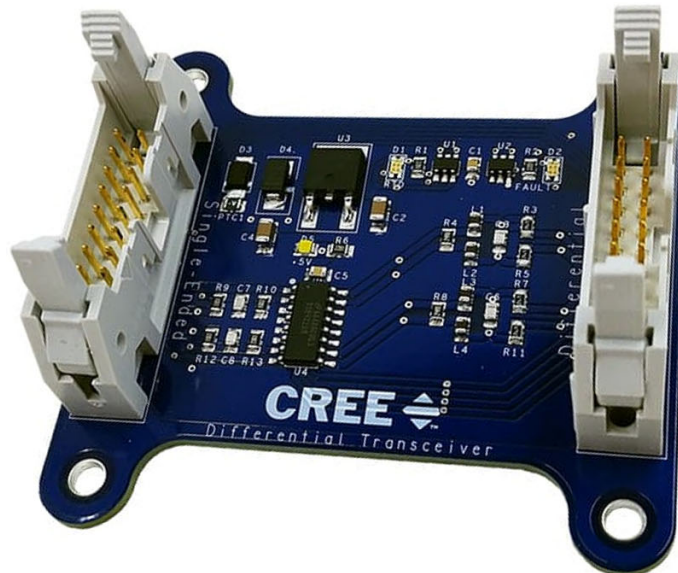
Figure 2. Functional Block Diagram and Differential Transceiver Daughter Card
