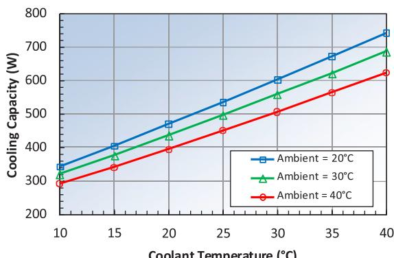
\*150 cfma airflow, 2 L/min w ater flow
