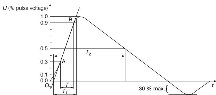
Front time:  $T_1 = 1.67 \times T = 1.2 \mu\text{s} \pm 30\%$
