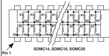
TTL dual-line terminator; pulse squaring, 12, 14, or 18 pairs of resistors
