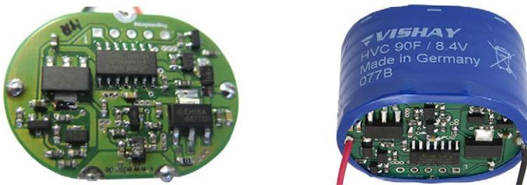
This version is optimized for a 196 HVC in a 90 F, 8.4 V configuration. Basically, it is a voltage converter and switch logic in one, which adjusts to a wide input voltage range. It provides the correct charging voltage and protects against deep discharge.
