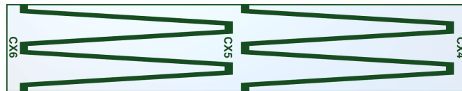
Figure 2.3: 3 Channel Slider with Touch Sensor Reference Schematic
