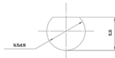
PANEL CUT-OUT DETAIL
