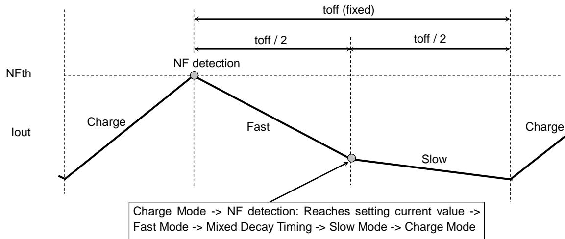
If the output current is zero-detected during Fast mode, the output becomes High impedance.
