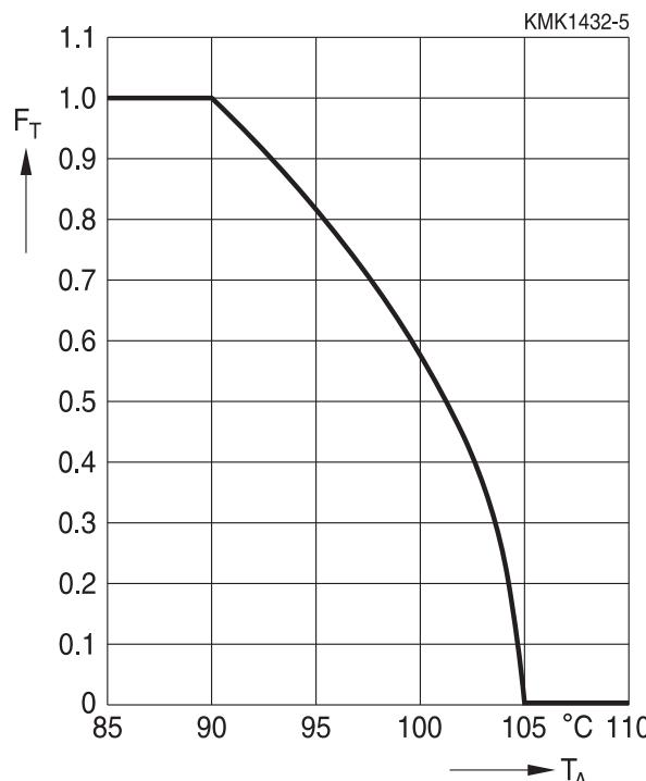
Maximum  $I_{RMS}$  current as function of the ambient temperature:  $I_{RMS}(T_A) = \text{Factor} \times I_{RMS}(70 \text{ °C})$
