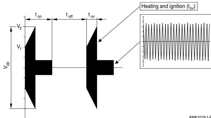
For a repetitive application of on/off switching pulses (as for example in the life tests applied by electronic ballast manufacturers), limits have to be imposed on the time periods under overvoltage and on the duty cycle, in order to keep the capacitance value within the required margins:
