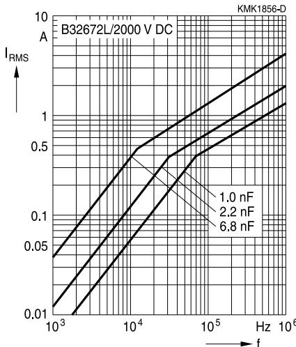
**Maximum AC voltage ( $V_{RMS}$ ), current ( $I_{RMS}$ ) versus frequency and temperature for  $T_A > 100$  °C**
