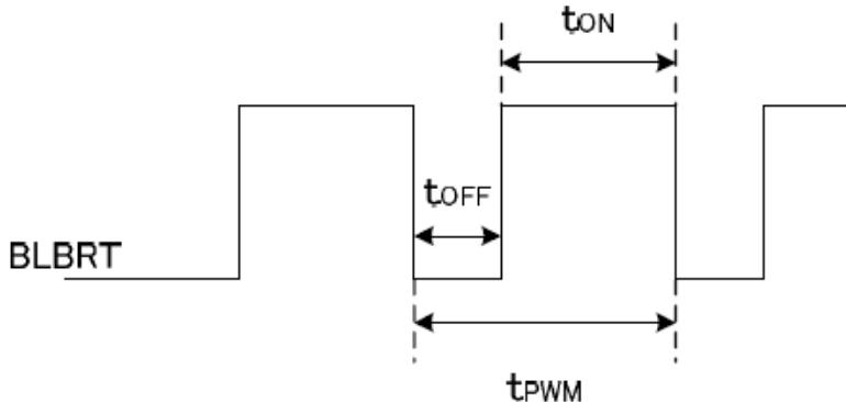
Please do not set  $t_{OFF}$  with  $0 \mu s < t_{OFF} < 1 \mu s$ .
