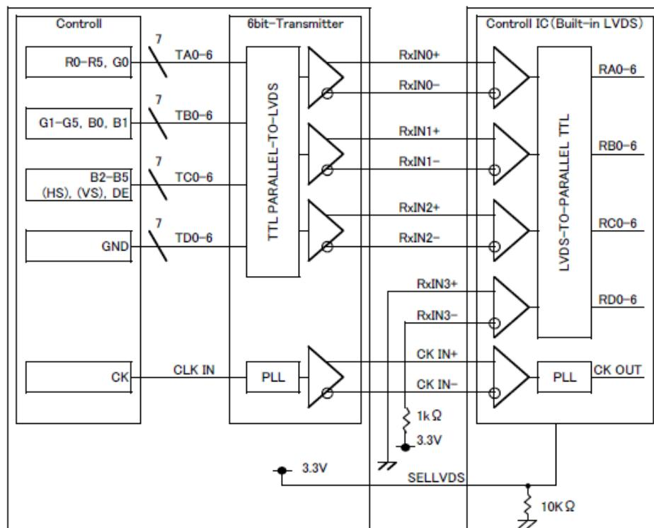
\*SELLVDS signal line has 10 k Ω pulldown resistor.
