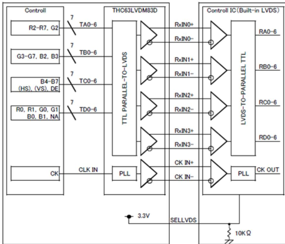
\*SELLVDS signal line has 10 k  $\Omega$  pulldown resistor.
