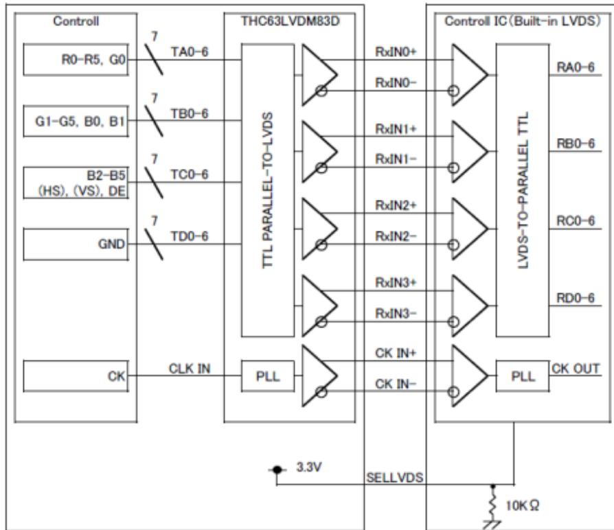
\*SELLVDS signal line has 10 k Ω pulldown resistor.
