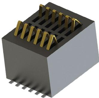
KYOCERA AVX has extended its range of board-to-board stacker connectors for connecting two PCBs with a new high version 00-9148. This new connector is designed to connect 2 parallel boards using a 1 piece connector design for 8mm board spacing in a double row configuration offering 8 positions at 1mm pitch. Rated at 1A continuous through each contact.
