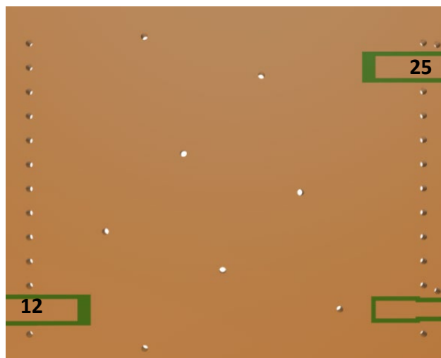
3D Image of Copper Clearance TFM.110A.
