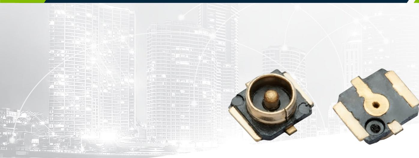
Part of the Taoglas SMD Mount Receptacle the RECE.20369.001E.01 is a 3-pad type wire-to-board SMD Receptacle solution that is ultra-small, lightweight and low profile (1.6mm MAX.) with an operational frequency range of DC to 8 GHz. Taoglas the RECE.20369.001E.01 is gold plated to have superior performance and allow easy mounting of the male RF connector.
