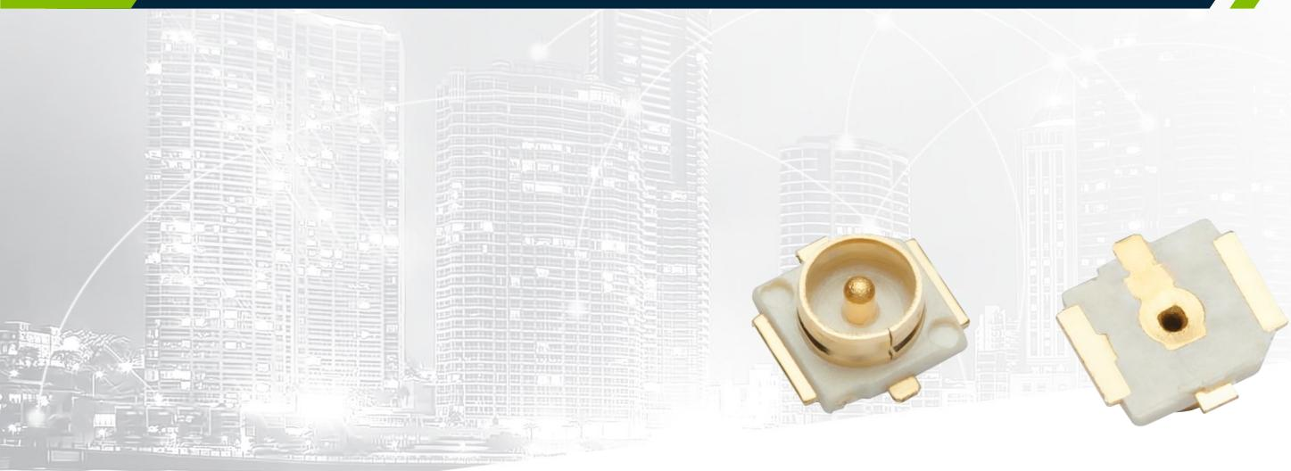
Part of the Taoglas SMD Mount Receptacle, the RECE.20279.001E.01 is a 3-pad type wire-to-board SMD receptacle that is ultra-small, lightweight and low profile, 2.5mm max. With an operational frequency range of DC to 8 GHz the RECE.20279.001E.01 is gold plated to provide superior performance and allow for ease of mounting with the male RF connector.
