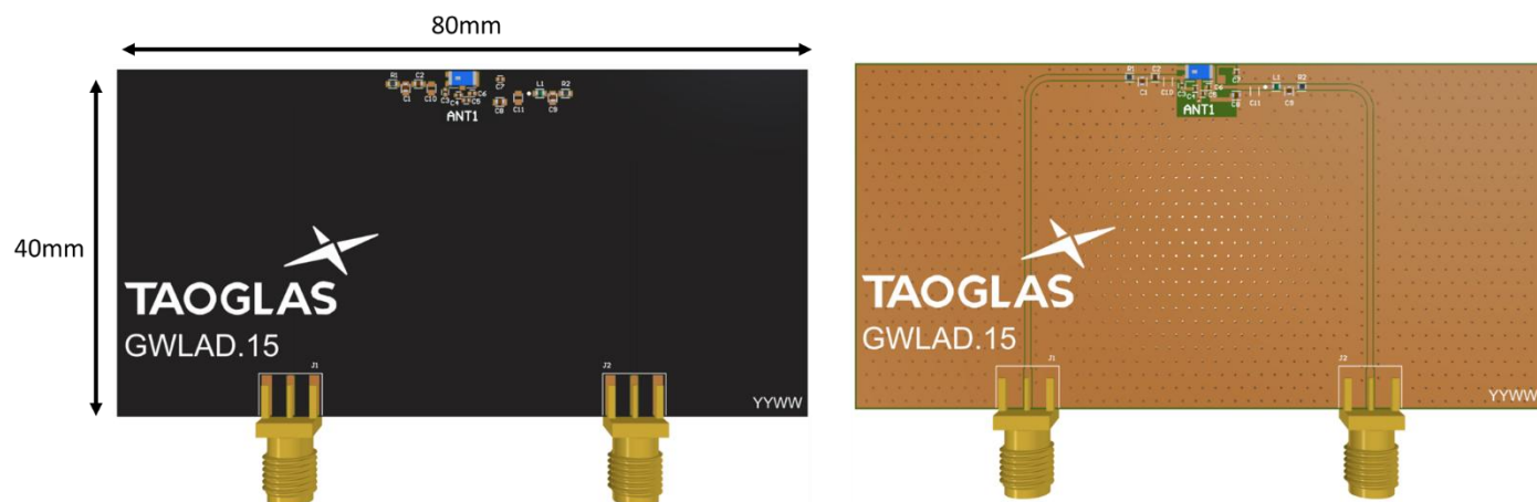
Top Side (GWLAD.15 placement on 80x40mm PCB)
