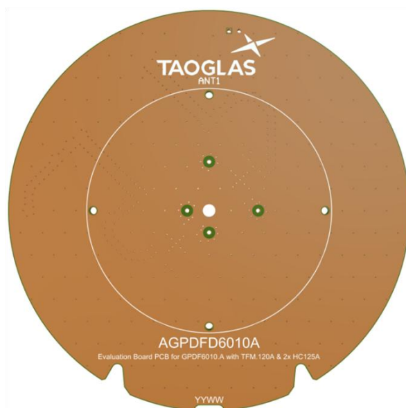
Top Side ( GPDF6010.A placement on 70x70mm PCB)
