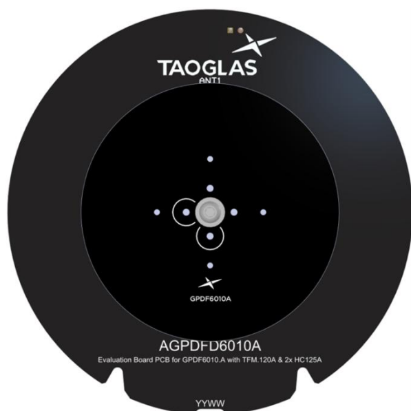
Top Side ( GPDF6010.A placement on 70x70mm PCB)
