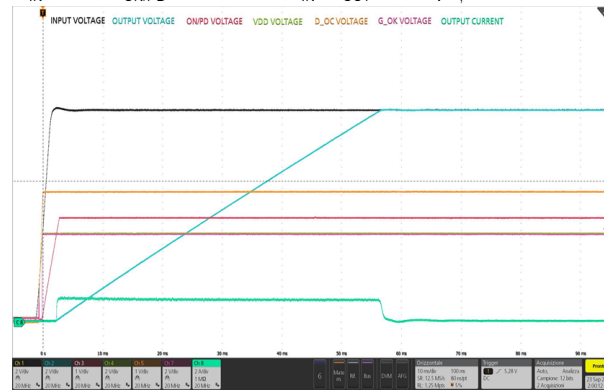
Figure 28. Startup by ON/PD (no load)
