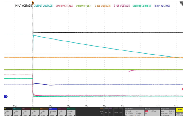
Figure 33. Output short-circuit during operation
