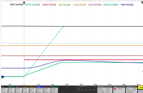
Figure 28. Startup by ON/PD (no load)
