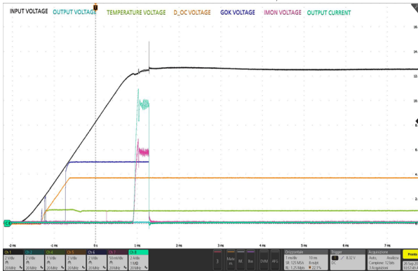
Figure 32. Startup into output short-circuit
