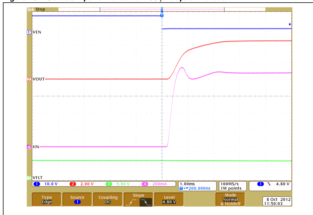
Figure 18. Soft-start performance for 100 \mu F capacitive load
