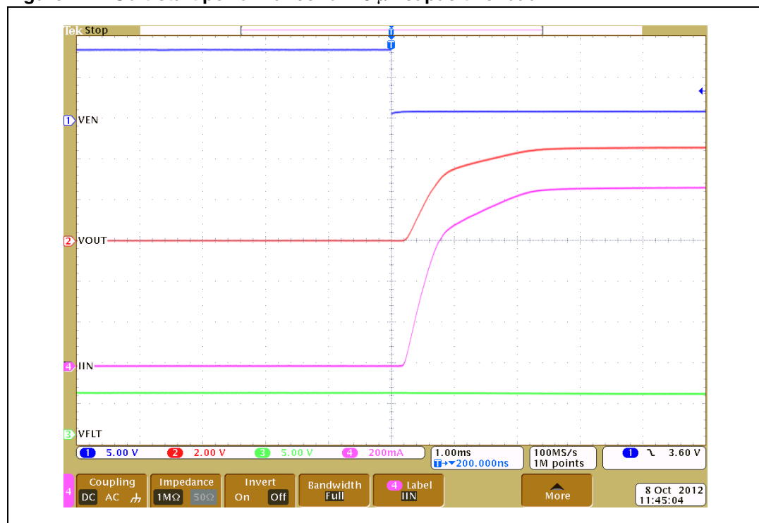
Figure 17. Soft-start performance for 10 \mu F capacitive load
