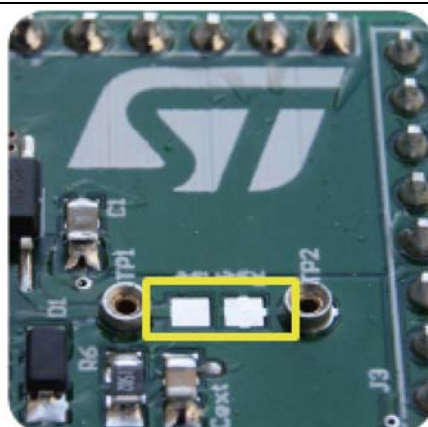
Figure 5. Pads for soldering SMD resistor
