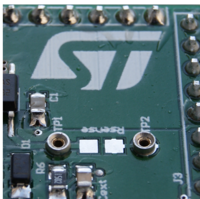
Figure 4. Mounting through-hole sense resistor
