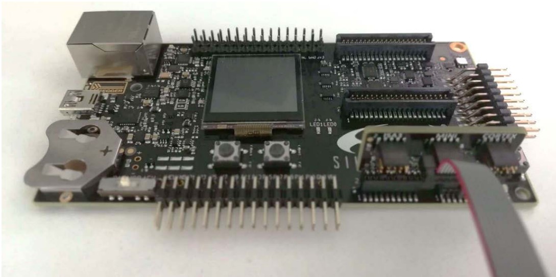
Figure 4.2 WSTK Board with STK/WSTK Debug Adapter Connected
