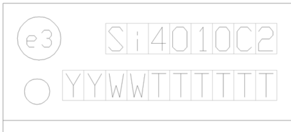
Figure 5.1. Si4010 Top Marking
