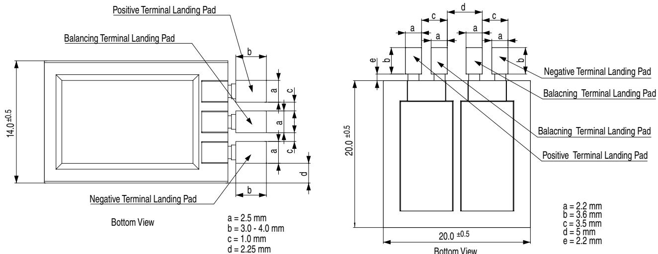
Soldering pads to Case TS20, TS22, TS32, TS35, FS37
