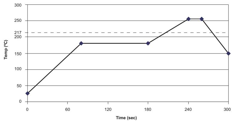
The recommended reflow profile is provided as a guideline. Optimal profile may differ due to oven type, assembly layout or other design or process variables. Customers should verify actual device performance in their specific application and reflow process. Please contact Piher if you require additional support.
