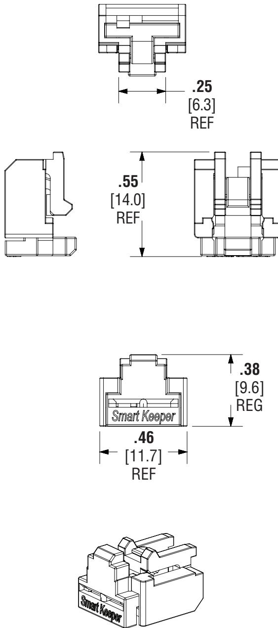
Dimensions are in inches. [Dimensions in brackets are metric].
