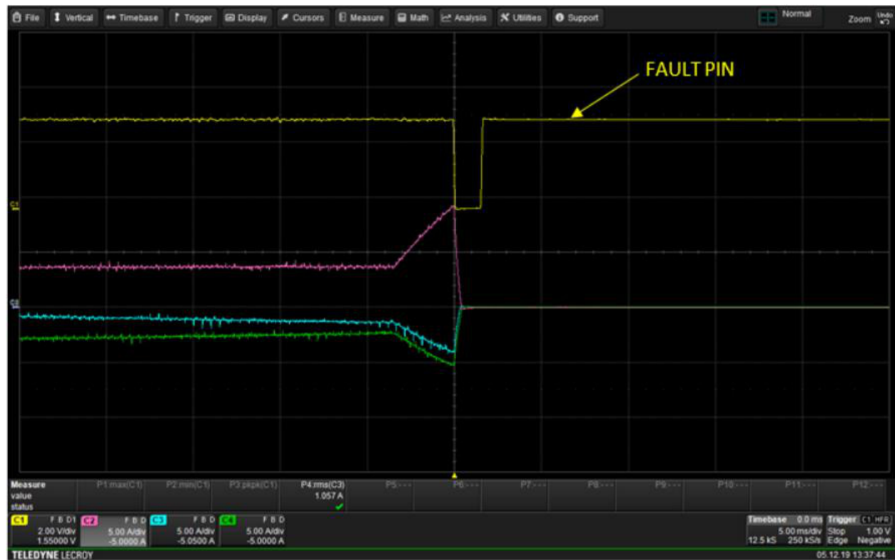
Figure 18. Reaction of Over-current Protection – Detail
