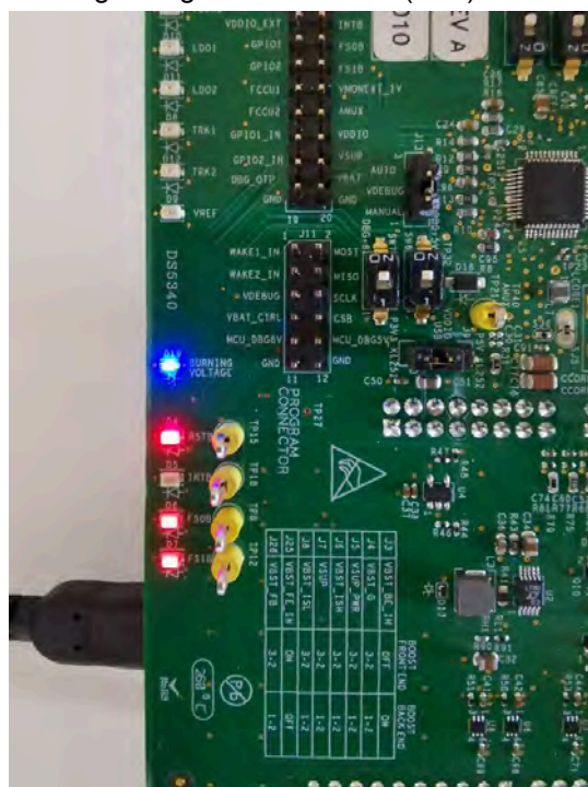
Burning voltage LED indicator (D19):
