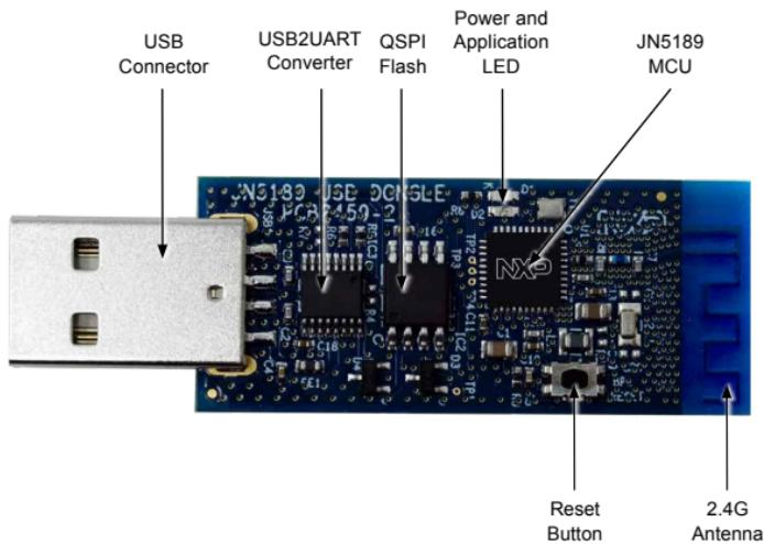
Figure 1: OM15080-JN5189 Board Components
