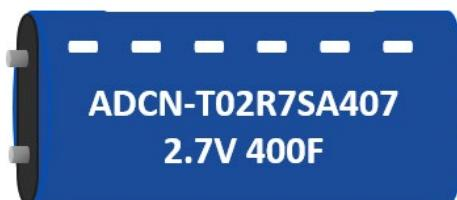
Example of the Markings of a 400F 2.7V capacitor
