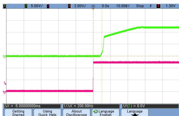
Output Ripple and Noise (Vin = 12V; Iout = 10A; Ta = 25°C; Cloud = 1μF ceramic||10μF tantalum||200μF Ecap; Scope BW = 20MHz)
