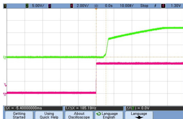
Transient Response (Vin = 12V, Vout = Nom, Iout = 50-75, Cloud = 1μF ceramic||10μF tantalum||200μF Ecap; Slew Rate = 1A/μs, Ta = 25°C)
