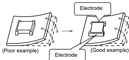
(2) Components location on PCB separation
