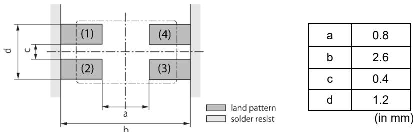
Do not use gilded pattern. A copper wire may cause open by dissolution of metallization.
