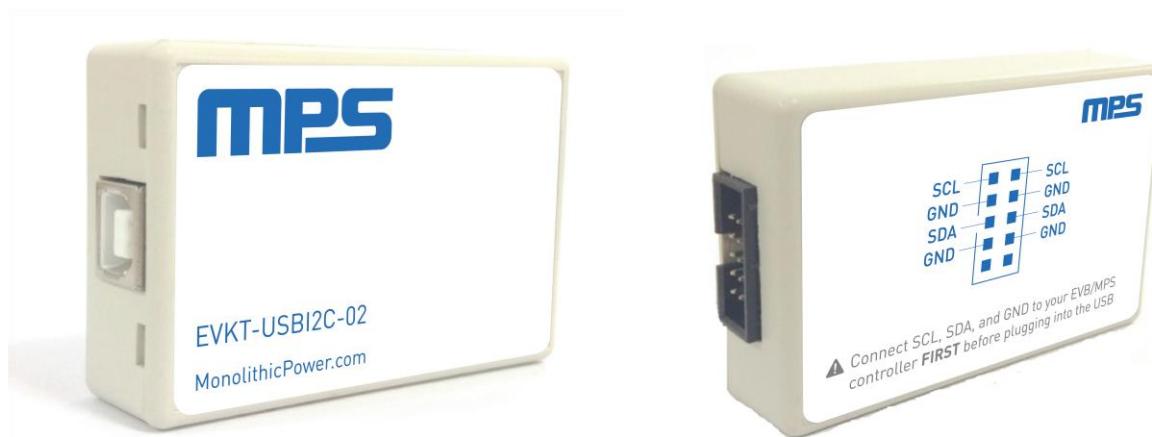
Figure 3: EVKT-USBI2C-02 Communication Interface
