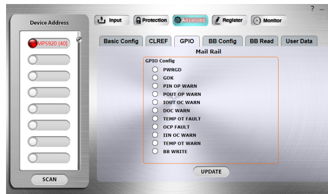
Figure 7: GUI Advanced Page, GPIO Tab
