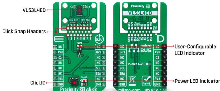
The VL53L4ED uses STMicroelectronics' FlightSense technology, allowing it to measure absolute distances regardless of target color or reflectance. It includes a SPAD (single photon avalanche diode) array, enhancing its performance across ambient lighting conditions and various cover glass materials. Additionally, the sensor integrates a VCSEL (vertical-cavity surface-emitting laser) that emits an invisible 940nm IR light, certified as Class 1 eye-safe.
