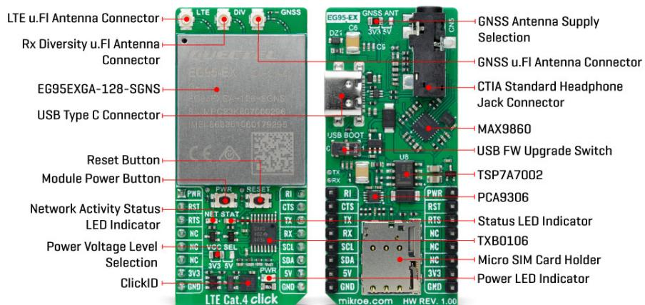
Communication between the EG95EXGA-128-SGNS and the host MCU is made through a UART interface, using standard UART RX and TX pins and hardware flow control pins (CTS/RTS/RI - Clear to Send/Ready to Send/Ring Indicator) for efficient data transfer. The module defaults to a communication speed of 115200bps, allowing for seamless data exchange over [AT commands](#). Notably, this module version also features an audio interface, which can be accessed via the I2C interface.
