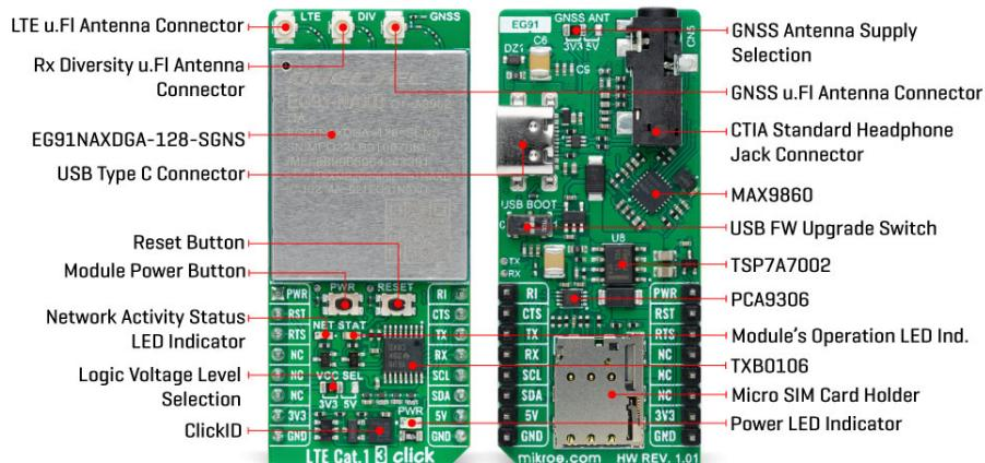
Communication between the EG91NAXDGA-128-SGNS and the host MCU is made through a UART interface, using standard UART RX and TX pins and hardware flow control pins (CTS/RTS/RI - Clear to Send/Ready to Send/Ring Indicator) for efficient data transfer. The module defaults to a communication speed of 115200bps, allowing for seamless data exchange over [AT commands](#). Notably, this telematics version of the module also features an audio interface, which can be accessed via the I2C interface.
