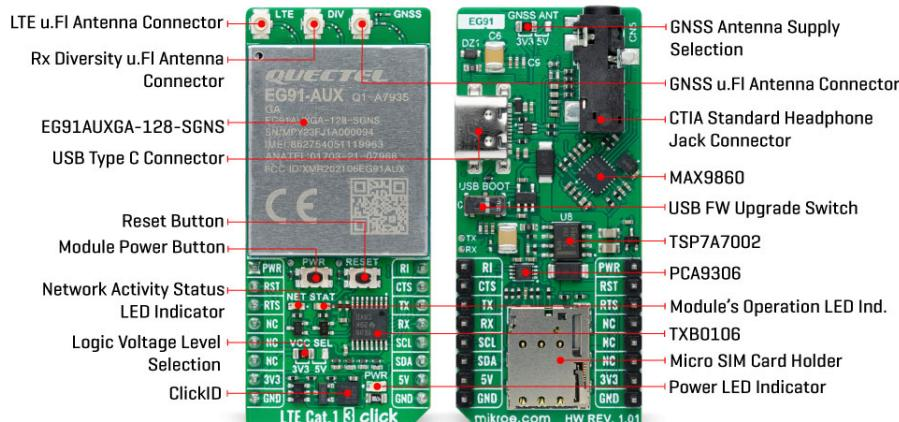
Communication between the EG91AUXGA-128-SGNS and the host MCU is made through a UART interface, using standard UART RX and TX pins and hardware flow control pins (CTS/RTS/RI - Clear to Send/Ready to Send/Ring Indicator) for efficient data transfer. The module defaults to a communication speed of 115200bps, allowing for seamless data exchange over [AT commands](#). Notably, this telematics version of the module also features an audio interface, which can be accessed via the I2C interface.
