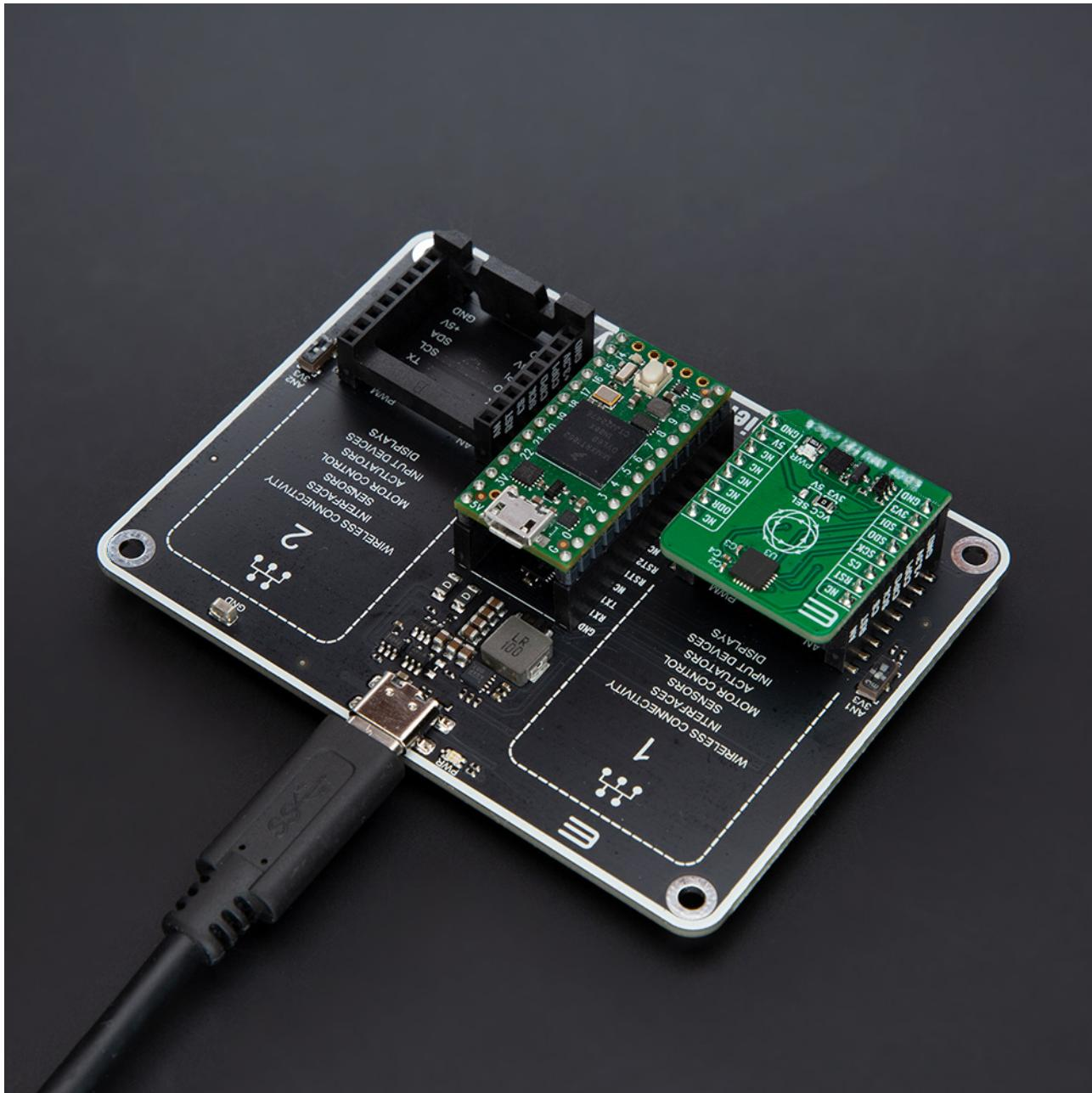
When the USB type C is connected to the Click Shield, the PWR diode will glow Blue, and at this setup, the connected Teensy 4.0 host board and all mikroBUS™ sockets will be powered from it.
