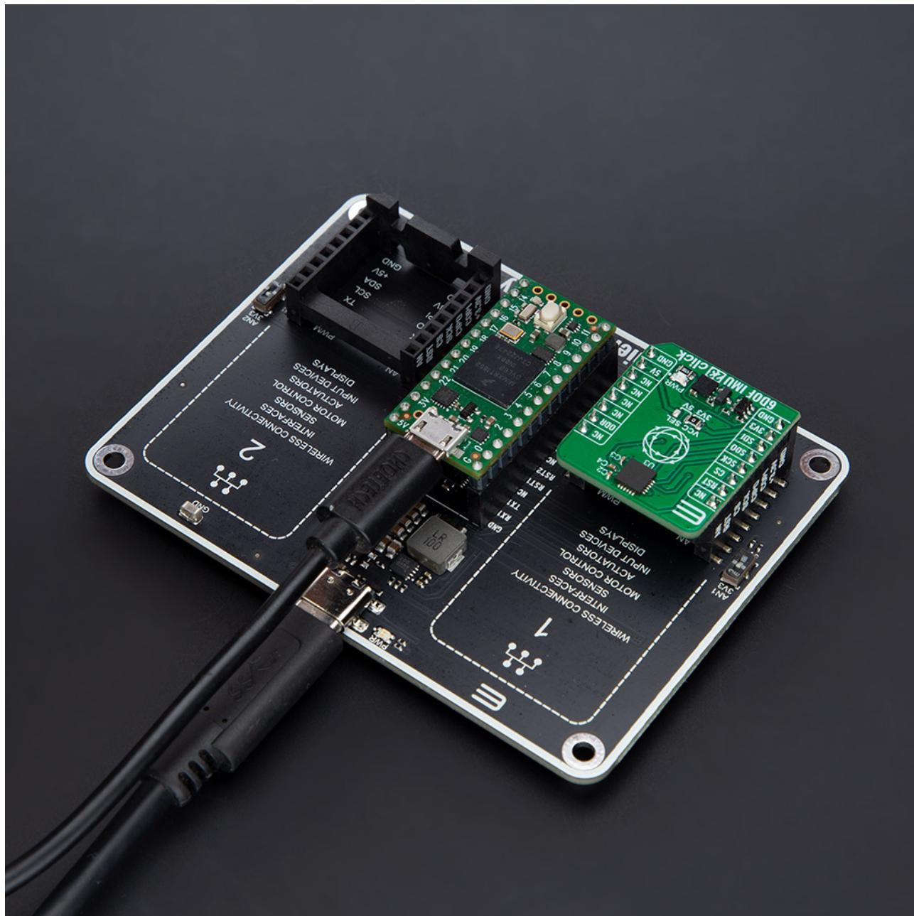
When the USB type C is connected to the Click Shield and the other USB is connected to the Teensy 4.0 board, the PWR diode will glow Cyan, and at this setup, the mikroBUS™ sockets are powered from the Click Shield.
