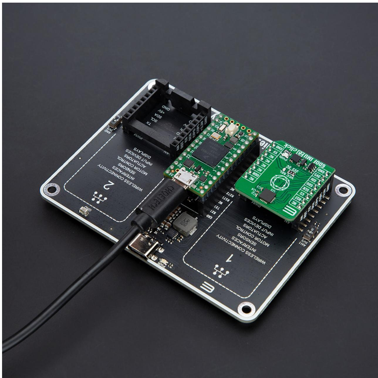
When the USB is connected to the Teensy 4.0 board, the PWR diode will glow Green, and at this setup, the Teensy 4.0 host board itself will be supplied, and it will provide power to the Click Shield, including all mikroBUS™ sockets.
