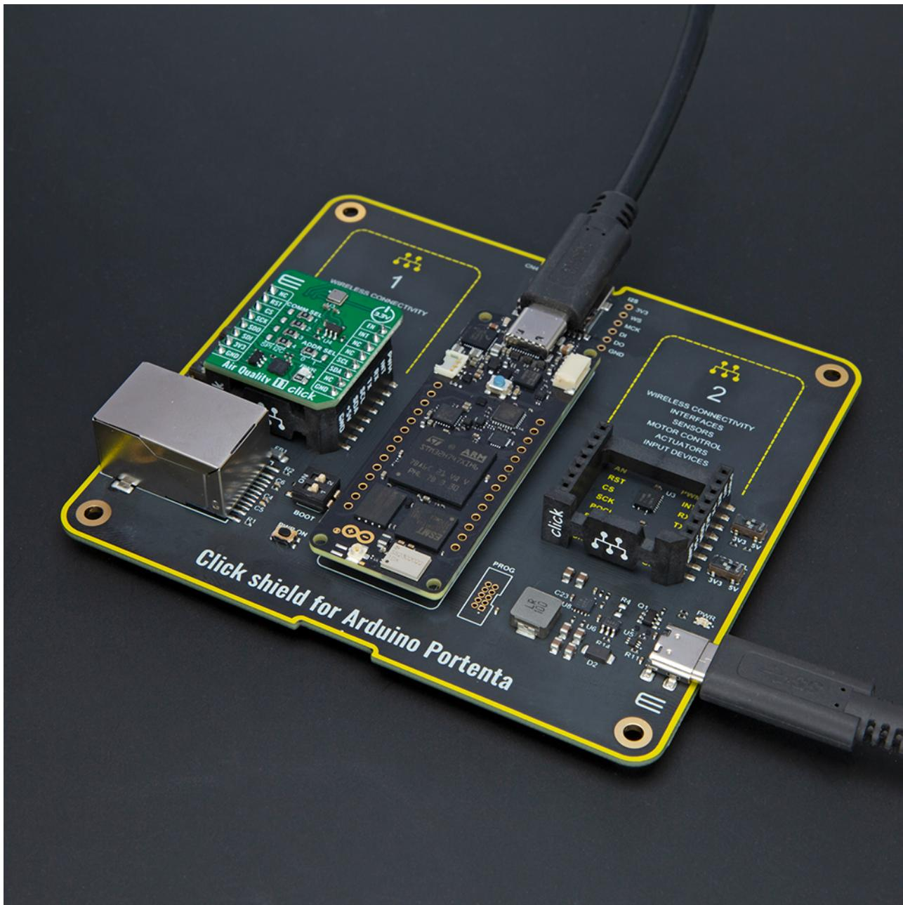
When the USB is connected to the Click Shield, and the other USB is connected to the Portenta board, the PWR diode will glow Cyan, and at this setup, the mikroBUS™ sockets are powered from the Type C connector from Click Shield.
