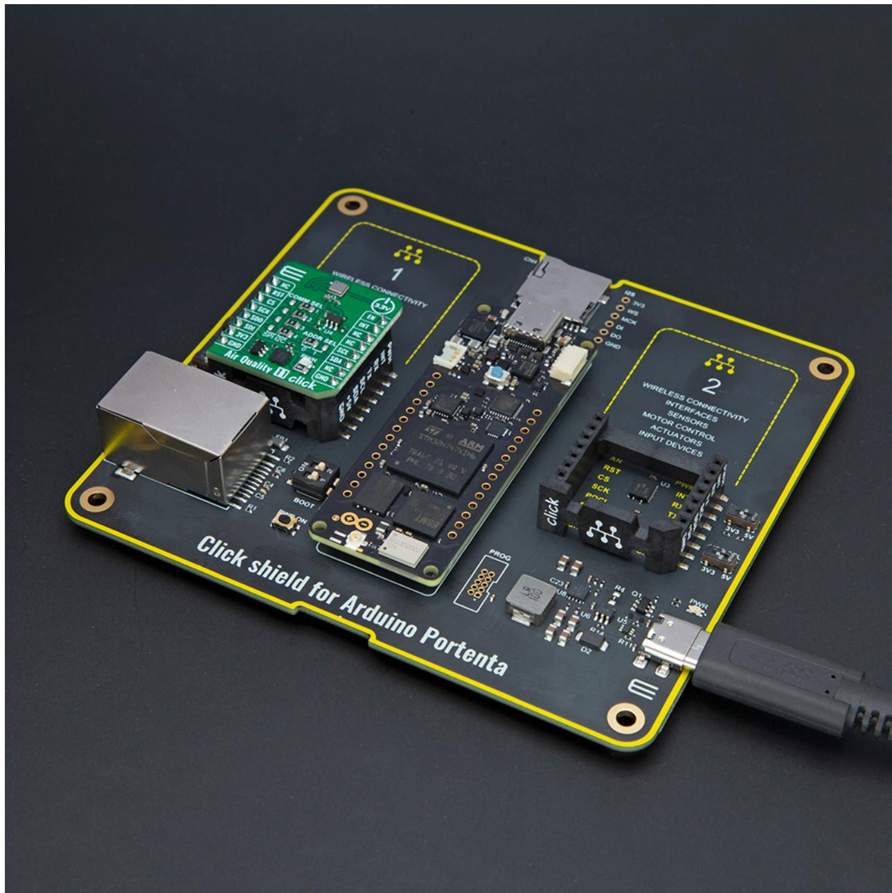
When the USB is connected to the Click Shield, the PWR diode will glow Blue, and at this setup, the connected Portenta baseboard and all mikroBUS™ sockets will be powered from it.
