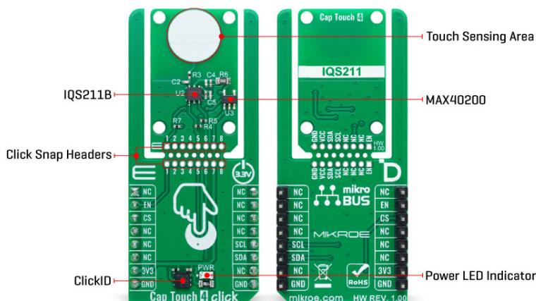
As mentioned, the IQS211B offers advanced features such as automatic detection and environmental compensation through its integrated finite state machine, eliminating the need for constant host MCU interaction. This allows for smooth operation without external interference. It also includes an integrated LDO regulator to enhance immunity against power supply noise, an internal oscillator for consistent performance, and built-in calibration capacitors to maintain accuracy over time.
