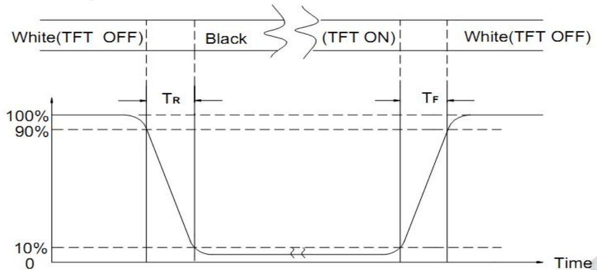
Note (5) Definition of Transmittance (Module is without signal input)
