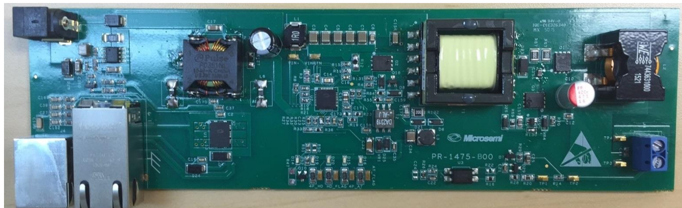
Figure 2: PD70211EVB72FW-12 Evaluation Board – General View
